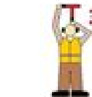
CONNECT TO GROUND POWER
