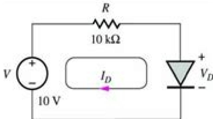
$V$  and  $R$  may represent the Thévenin equivalent of a more complex 2-terminal network. The objective of diode circuit analysis is to find the **quiescent operating point** for the diode.
