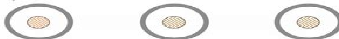
Figure 5.1 - Layout of three, single-core cables
