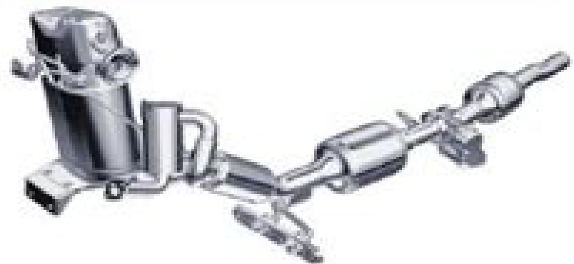
2.0 Liter TDI Common Rail Engine with Clean Diesel System
