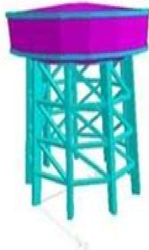
Fig.3 Model of Intze type water tank With Diagonal Bracing
