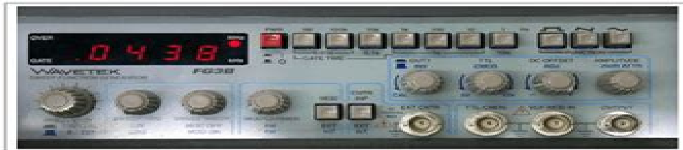
Figure 2.1 Front panel of Wavetek FG3B function generator.
