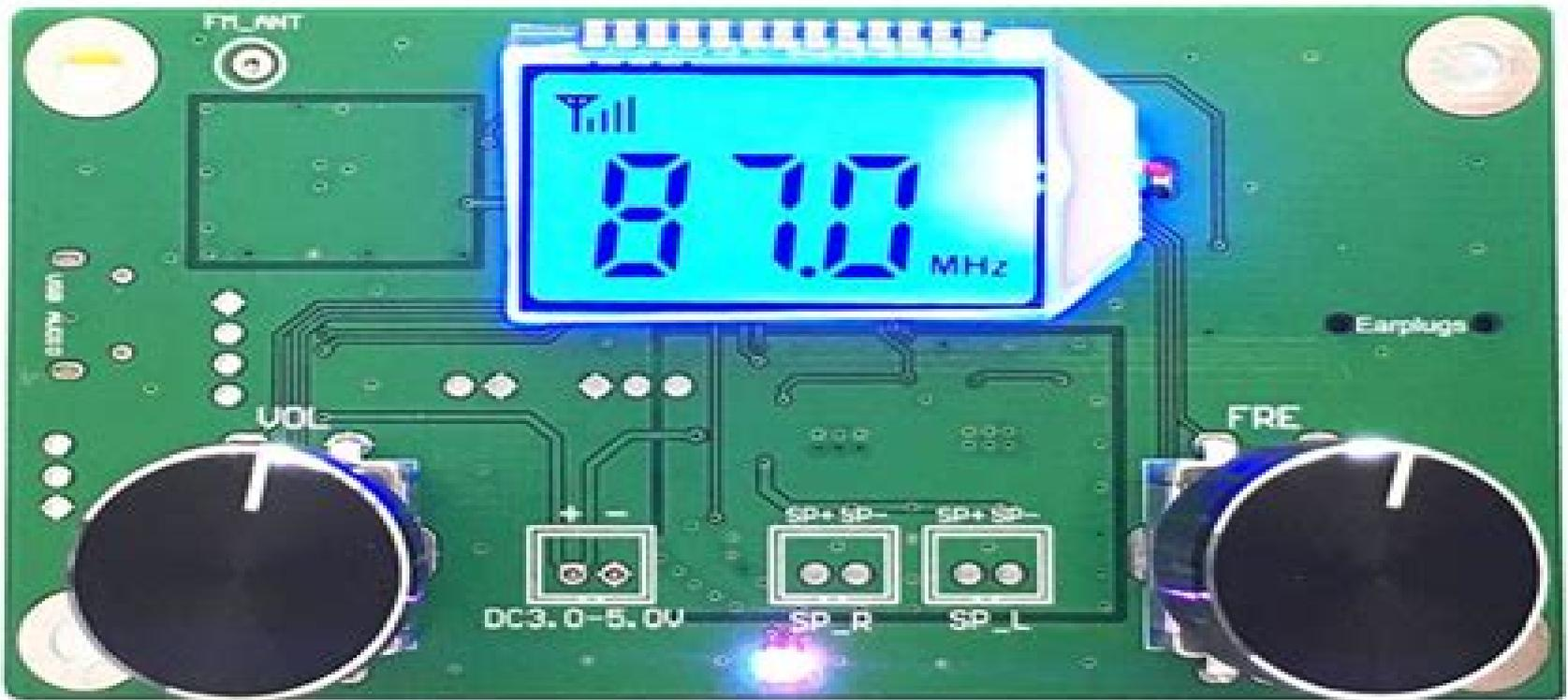
**Digital Stereo Radio Dsp Pll Fm Receiver Module 87mhz**
